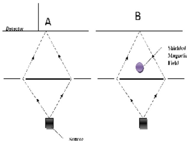
**Fig. 2.** Aharonov-Bohm effect: In the interference experiment for electron particles, in part A there is no any magnetic field around the set-up, but in part 2 there is a shielded magnetic field after the two-slit which has no any classical effect on the paths of electrons. The interference representations on detectors A and B are different. The magnetic field in part 2 has changed the wave phase of electrons.
